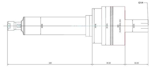
FDT is an air driven flexible tool that follows the undefined edges on the workpiece.
